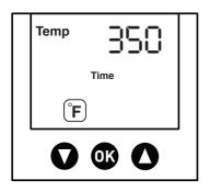
**4.** After temp setting, press the button to enter time setting. After time and temp is set. Press the button, and the machine will start heating.
